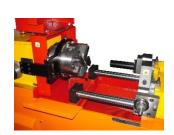
The grinding machine allows a rapid sharpening of the chasers and guarantees the good cutting angles of your chasers, depending on the hardness of the metals you must thread.
